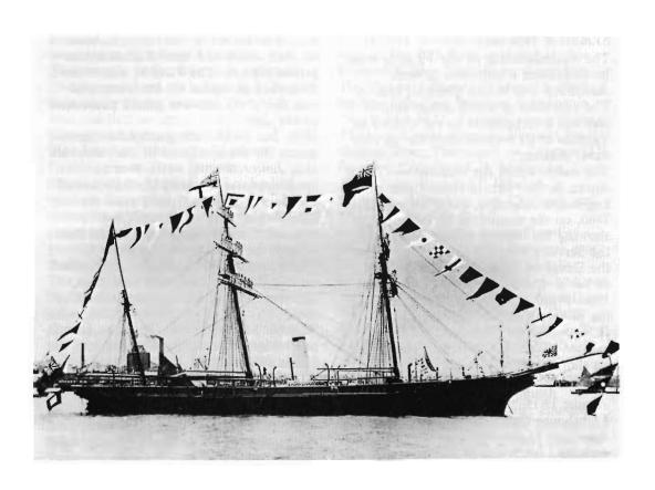
"Specifications for building a Screw Steamer Vessel to be named the "Victoria" of the following dimensions; "Length between the perpendicular 166 feet, keel for tonnage 149 feet 9½ inches, breadth extreme 27 feet 2 inches, breadth for tonnage 27 feet depth in hold from lower side of deck to upper side of skin 16 feet, burden in tons no. 580, ...".
