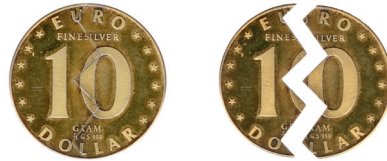
Figure 5. Example of wire erosion jagged line cut through sample Euro coin.
