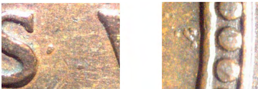
Figure 8A. Die markers from rust.
