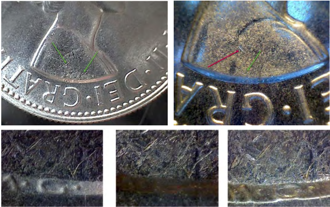
Figure 2 Reveals the obverse shoulder and undamaged rim area of two proof 1963 florins and below at higher magnification are a strip of microphotographs under different lighting of the truncation area for the upper left coin. The two upper pictures reveal obvious scratches as per the red arrow were a scratch diagonally crosses over the tunic's seam. The green arrows highlight irregular surface marks, which are the focus of this article.
