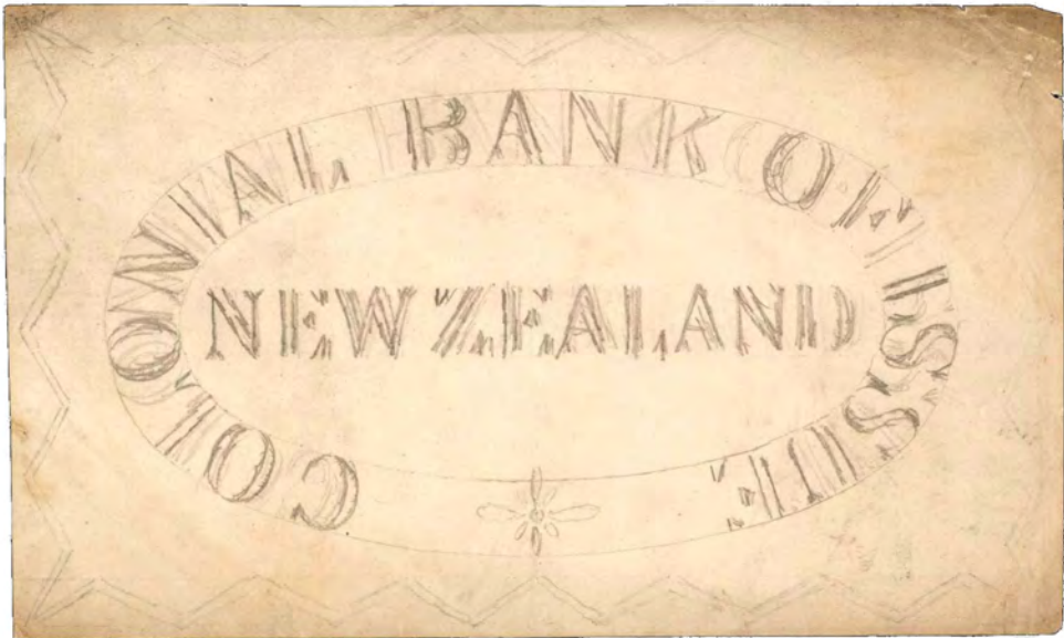
Fig. 3 Perkins, Bacon & Petch essay for the watermark design on the Colonial Bank of Issue £1 and £5 notes, ca.1849. This design was engraved into relief, then transferred to a fine wire mesh and used during manufacturing to impress a watermark onto wet paper sheets. [Image A. Clifford]
